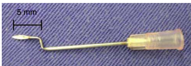
Fig. 2 – Needle preparation to perform the puncture. The final 5 mm of a 40 mm × 12 mm (18 G 1/2) needle was delimited from its bevel and folded in an S-shape in order to standardize the depth of the punctures.
